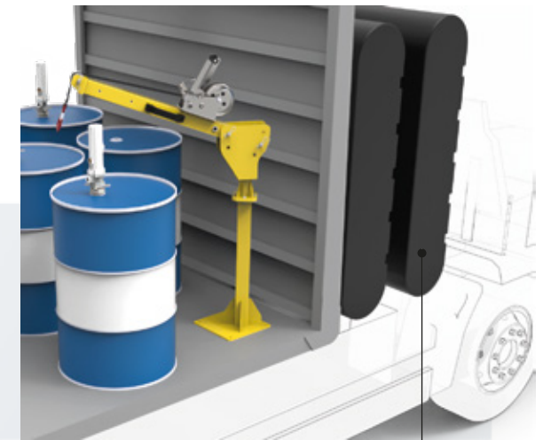
Tanques de gas oil 950 lts x 2
